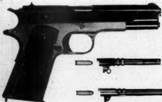
Mr. Kirby's 9.8 mm. Colt is strikingly similar to other Colt automatics, but the slide, barrel and barrel bushing are especially made for it. At right are (above) 9.8 mm. and (below) .38 ACP cartridges and barrels
